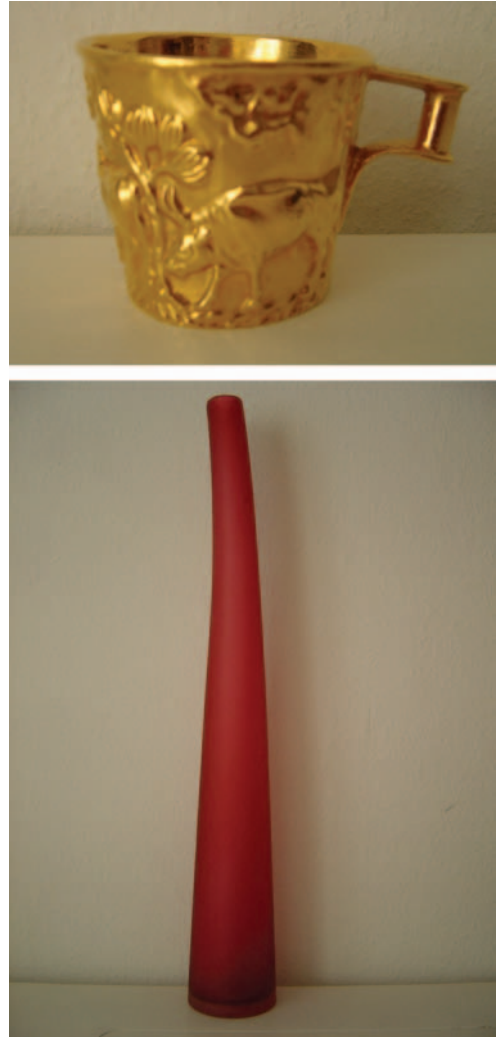
Figure 2. The colour of metallic gold and of gold nanoparticles in ruby glass.
